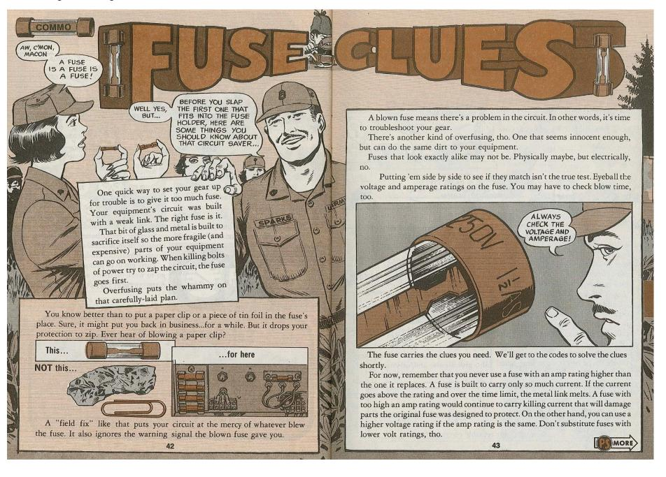
When that fuse link melts, electricity can still arc across the gap. The link finally melts away, creating a gap too wide for arcing. Before the gap widens, electricity continues to arc. The voltage rating is the most volts the fuse will take without arcing over. Too low a rating, and arcing keeps the circuit closed. If in doubt about which fuse your
